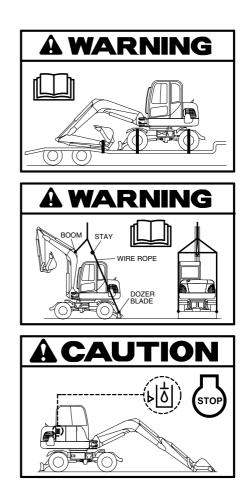
**18) GENERAL WARNING-FRAME** (item 21) This warning label is positioned on the right side window of the cab.
